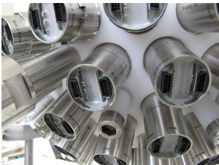
Figure 3: Back side of the reservoir, the transceivers are placed in cylindrical cases ("heads")
