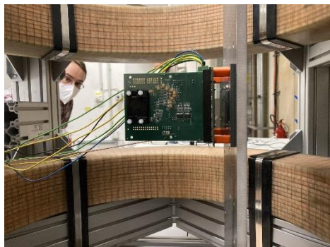
Figure 8: Sensor test in magnetic field
